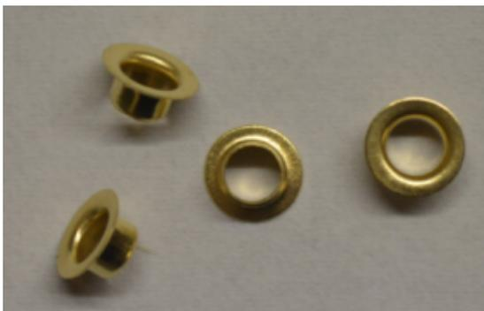
Locate the 4 brass bearing inserts and press them into the holes on the inner bogie frame.
