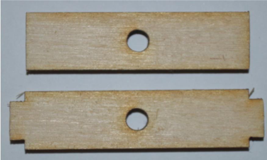
Locate the 2 parts which make up the frame spacers. The part without the tabs is the upper spacer.
